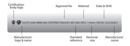
The Swv pipes fitting has been clearly and durably marked by moulded impression for each cavity of products.
